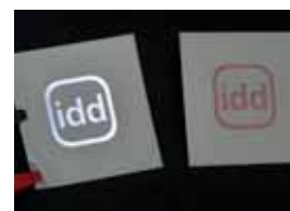
Screen printed electroluminescent panels produced at IDD which consist of up to seven layers of different functional inks.
