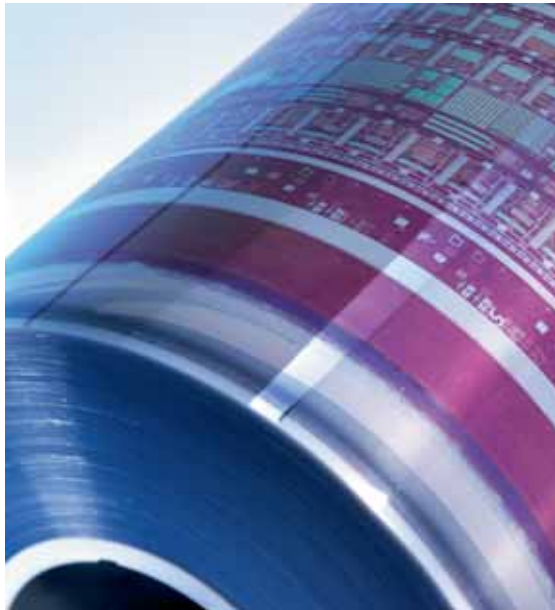
Printed electronics on roll produced by PolyIC
