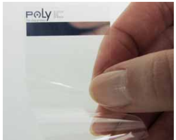
Transparent, conductive structures with a customized layout on thin, flexible film
