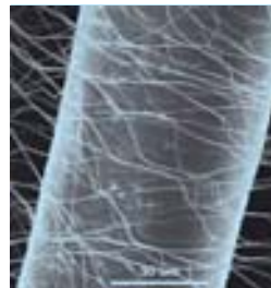
Tiny, hollow, porous, and incredibly varied: nano-fibers from the University of Marburg under an electron microscope (horizontal) as compared to a human hair (vertical)
