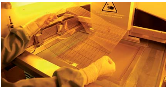
Printed organic CMOS circuits developed and produced by CEA / LITEN
